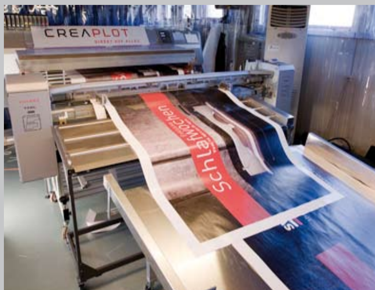
Interface between plotter and cutter. Optional dryer unit for solvent Ink.
