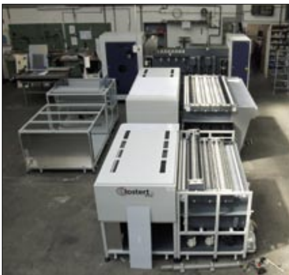
A new Hostert Pro LL (in the foreground) is being assembled, and a second-hand one (in the background) is being refurbished. The more compact design of the new machine is very striking.
