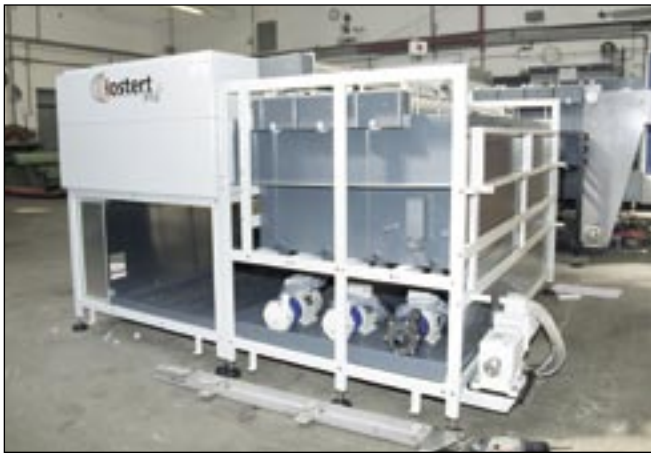
Apart from the sheet metal working, all machine parts are made in-house. This picture shows a new Hostert Pro LL, assembled by hand.
