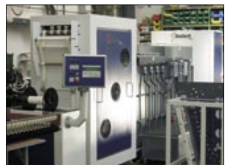
The Hostert Pro roll-paper machine HP-RP 12 with leaderband transport was introduced in 2004. All the dryer systems have been thoroughly revamped and the racks significantly improved.
