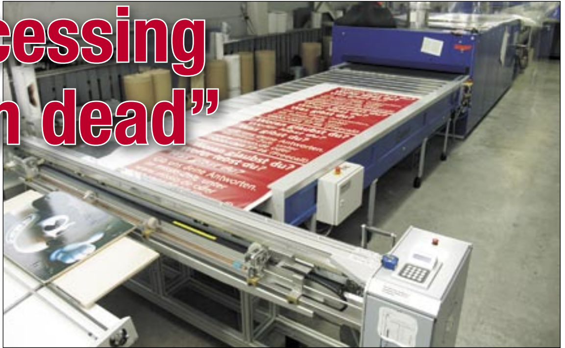
The feed and alignment unit for the graphics segment is one of the latest developments to come from Hostert Pro. It is installed with large-format inkjet printers between the dryer and the cutting unit to ensure that large-format prints can be cut fast and economically.
