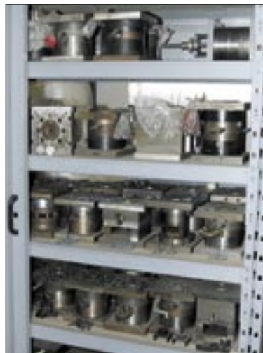
The injection molds for all the plastic parts ever produced by Hostert and Hostert Pro are stored in several cabinets.
